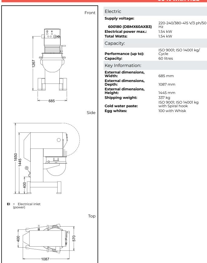
Planetary Mixers Stainless Steel Planetary Mixer, 60 It with Hub
